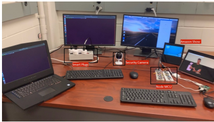
Figure 4: Testbed setup consisting of IoT devices such as smart plugs, Amazon Echo Show, laptops and computers.
